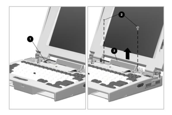
Figure 5-28. Removing the Status Panel
